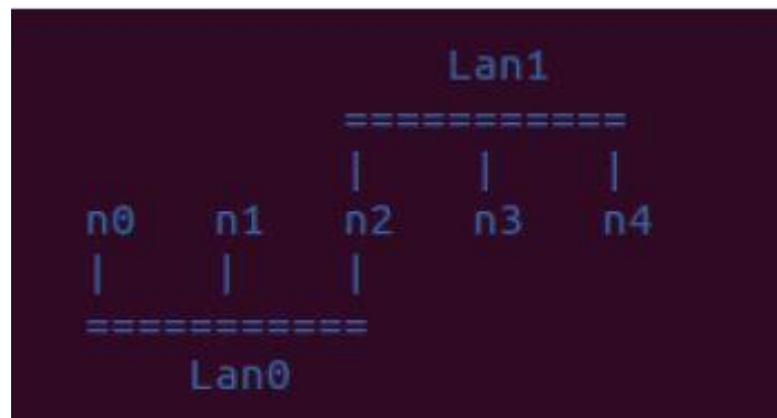
Figure.6. Default Multicast Topology
